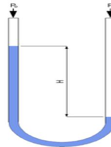
The difference in fluid height in a liquid column manometer is proportional to the pressure difference.
